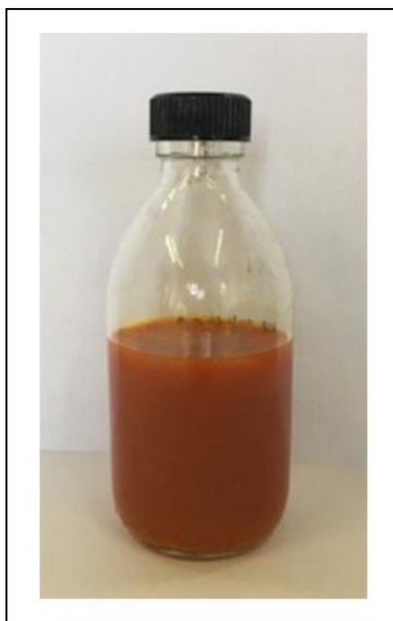
Figure II - 1: Template colloidal dispersion of Sn x Sb y S z in DMF.
