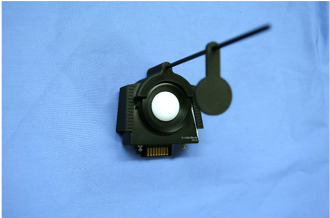
Fig. 8. Shroud and baffle rod assembly mounted to the T10A sensor head
