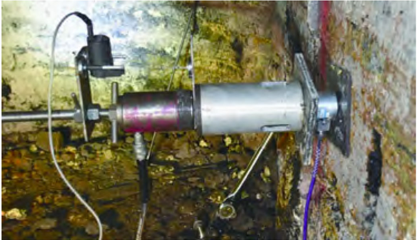
Fig. 5. Pull-out test gear mounted on the tested bolt.
