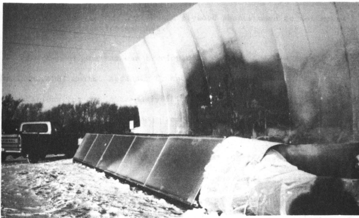
Figure 10. Frost accumulation on reflector and collector surfaces. Melting usually was completed at approximately 0900 h.
