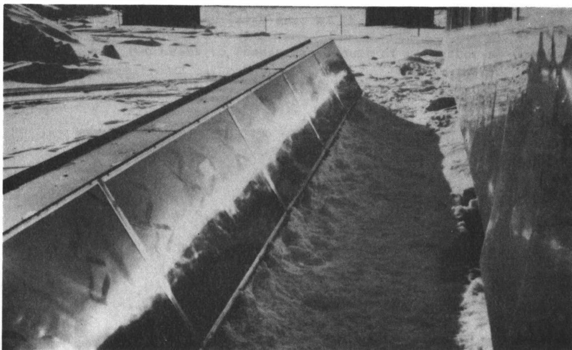
Figure 9. Concentrated band of solar radiation focused on the north collector by the concentrator. Note the glass cover framework, metal top cover, and collector baffles.
