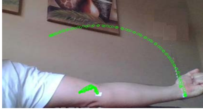
Figure 1. Captured image showing the author's experimentation with the computer vision tracking algorithm on his elbow joint at-home while describing the lab module to students in an online delivery mode.
