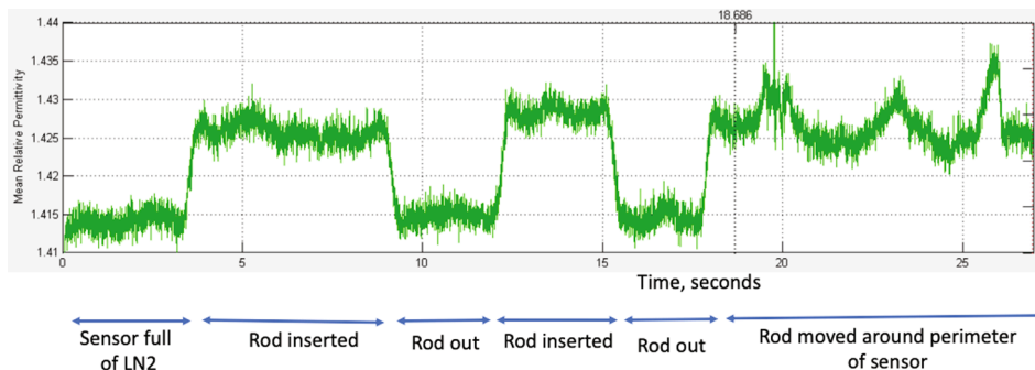
Fig. 11. Rod insertion tests - mean permittivity against time.
