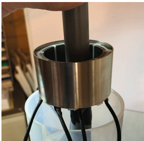
Fig. 6. Plastic tube filled with polypropylene beads being inserted into sensor.
