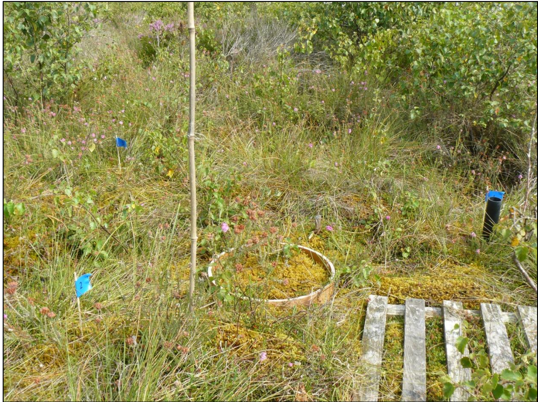
Figure 4.1. An example of the experimental field set up for one sampling point for GHG flux monitoring (collar), three microbial plots (blue flags) for the collection of a composite sample from each sampling point and measurements of water table position (black dipwell).
