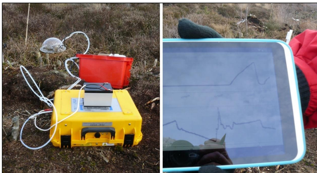
Figure 4.2. Field equipment at the youngest restoration area (RES6YRS). Los Gatos GHG analyser and chamber (left) demonstrating real-time fluxes of CO 2 and CH 4 (right).
