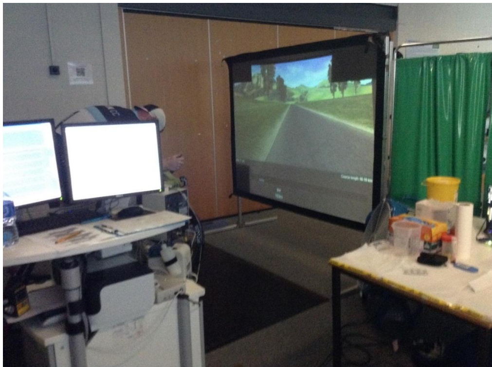
Figure 3.1 Positioning of 230 cm screen 130 cm away from the front wheel.
