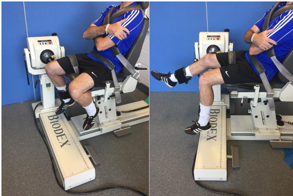
Figure 3.1. Figure 3.1: Experimental set-up for Isokinetic Dynamometry Testing.
