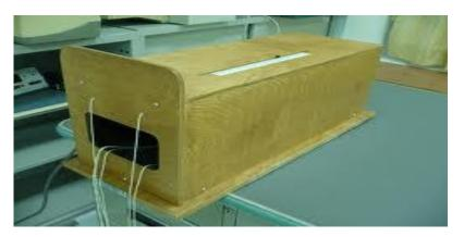
Fig 3.4: Lafayette Instrument Depth Perception Apparatus
