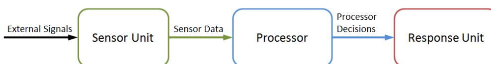
Figure 2: Block diagram of the child heat injury prevention system (Ferrara et al., 2013)
