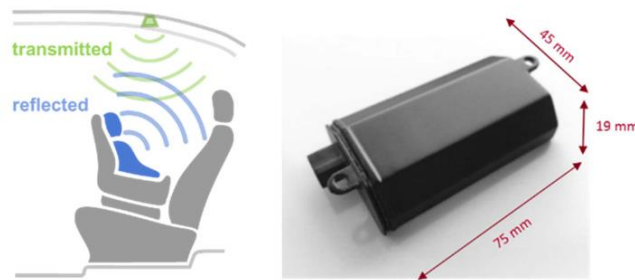
Figure 6: Radio-frequency based system sensor location (Mousel et al., 2017)
