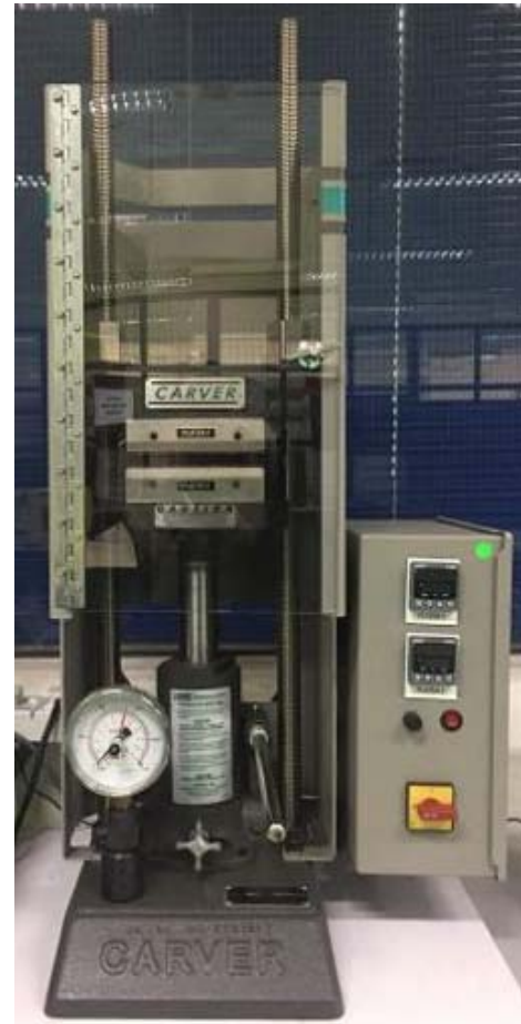
Fig. 2. Hydraulic laboratory hot press machine
