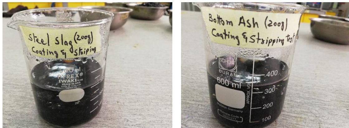
Figure 2. Coated specimens of SS and BA immersed in distilled water.
