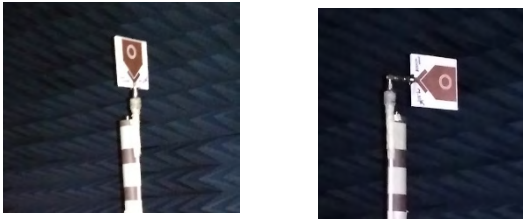
FIGURE 7. Measurement setup of the CP/LP-antenna in an anechoic chamber.
