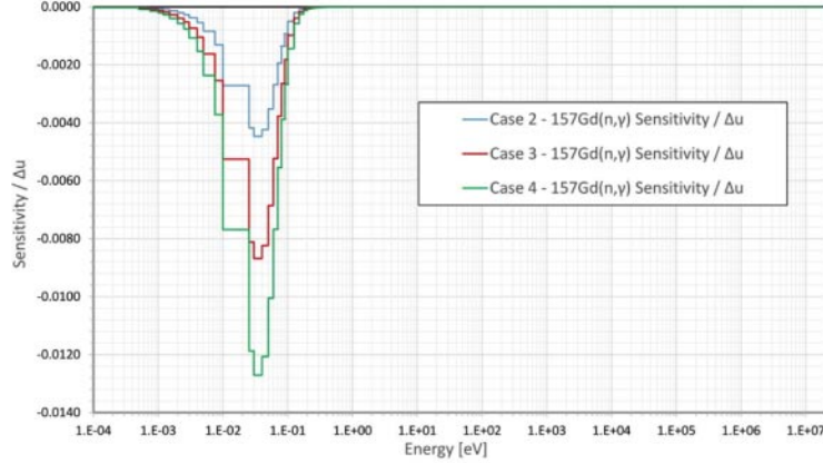
Fig. 2. – ZED-2 k_{\text{eff}} sensitivity per unit lethargy to ^{157}\text{Gd}(n,\gamma) .
