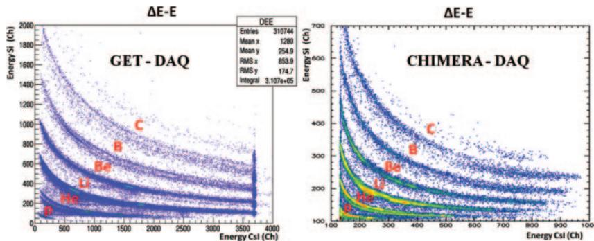
Fig. 2. – Two  $\Delta E$ - $E$  identification matrixes obtained from the same telescope with GET Electronics (left panel) and the standard CHIMERA acquisition (right panel). We used fragmentation beams at 50 AMeV on a plastic target in both experiments.
