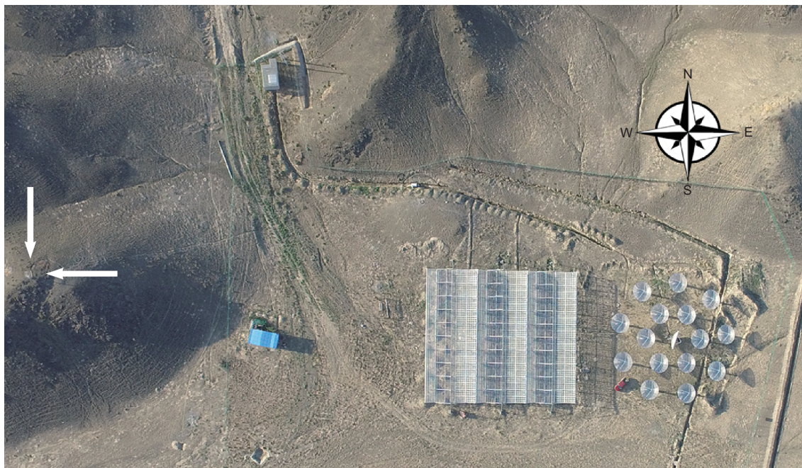
Figure 1 A top view photograph of the Tianlai cylinder and dish arrays. The dish array is located on the east side of the cylinder array, and the calibrator noise source (CNS) is located on a hill to the west of the arrays, as marked on the left side of the photograph. There is a blue cabin for storage between the array and the CNS.
