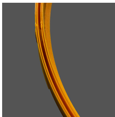
Figure 11. Walls not touching.
