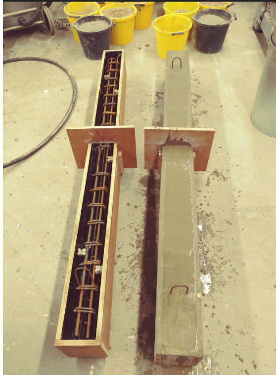
Fig. 3: Beam concrete casting
