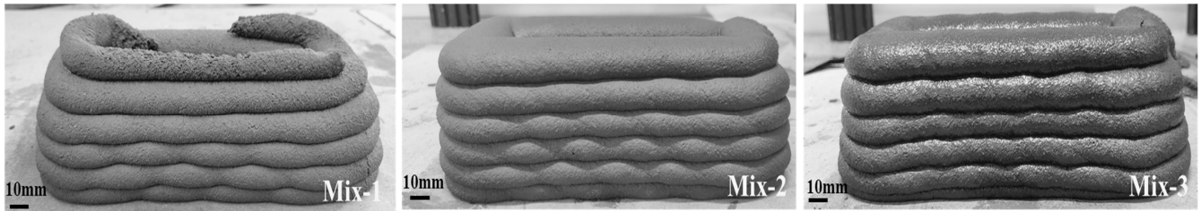
Figure 11 – Shape-retention ability of geopolymer composites.
