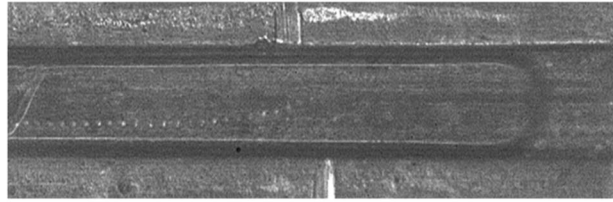
(b) Slug flow in TS2, q'' = 157.2 \text{ kW/m}^2 , G = 400 \text{ kg/(m}^2 \text{ s)} , x_{local} = 0.031 , \beta = 2.56
