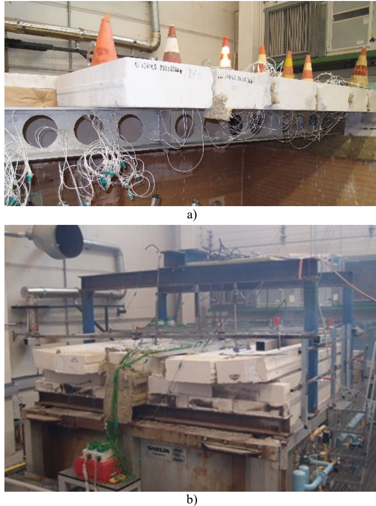
Fig. 2. a) Beam and slab construction during installation; b) Test set-up during the test.
