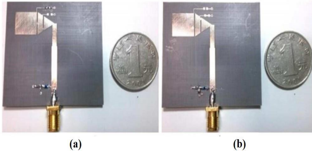
Figure 2.11 Bow-tie antenna with multiband frequency using PIN diodes at (a)2.4 GHz and (b) 3.5 GHz [53].
