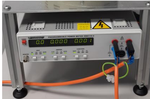
Figure 3.12 Photograph of power meter.
