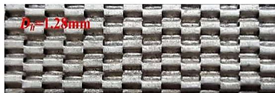
Figure 2.32 Photograph of serrated fins multi-channels with 1.28mm hydraulic diameter, Wen et al. (2019).
