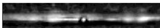
Figure 2.18 Nucleating bubble in the liquid film of annular flow, Borhani and Thome (2014).
