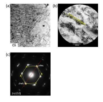
Figure 3. TEM micrographs at the early recrystallization stage of (a) ZW01 sheet annealed at 350 °C x 3 min. (b) Dislocation structures and (c) formation of a strain-free grains inside micro-bands observed in the W1 sheet annealed at 350 °C x 1 min. Note that the SAED of the area 'B' shows a similar orientation relationship with that shown in Fig. 2 (c).
