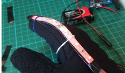
Fig. 4. LED strips and flex sensors embedded in initial prototype.
