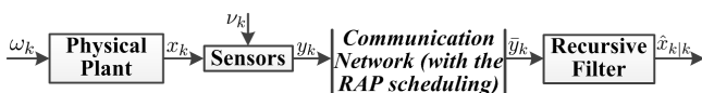
Fig. 1: Schematic structure for the plant and the filter over a network (with the RAP scheduling)
