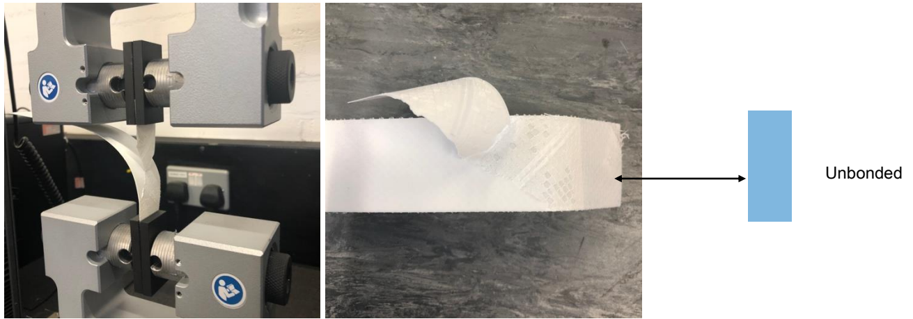
Figure 8: The delamination of PLA-F3 sample.
