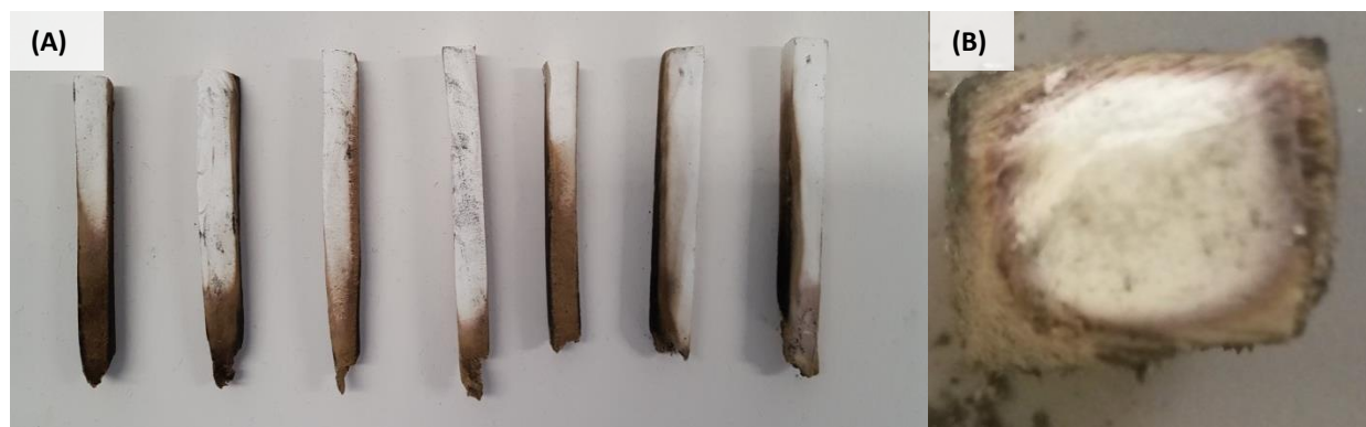
Figure 9.8 (A) Samples CR1-WR 0.5:2 after UL94 test (B) Cross-section of burned aerogels
