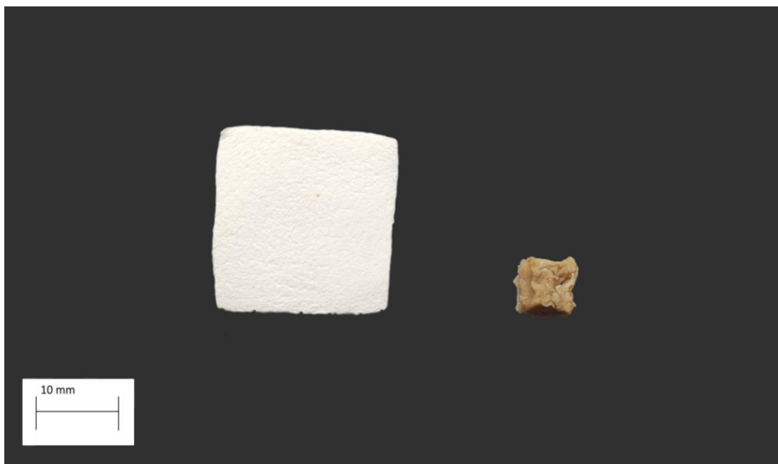
Figure 9.5 Shrinkage of the sample after 30 days in water: Sample CR1/WR1:2 shrunken by 6 % (Left) and Sample 0.3WR shrunken by 92% (Right)
