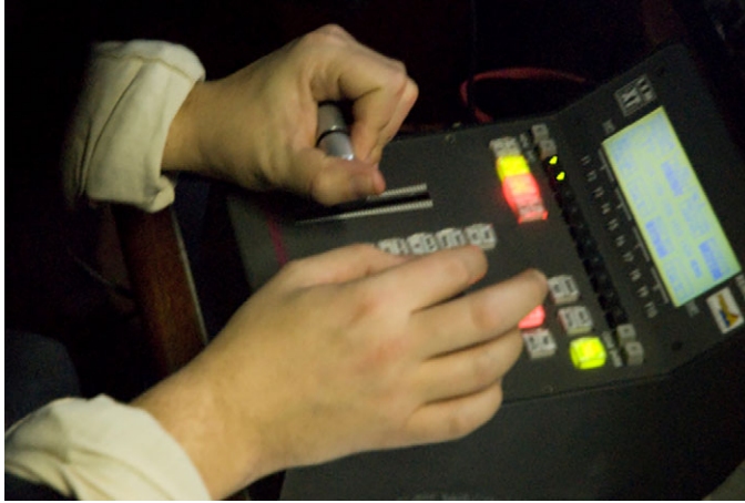
FIGURE 5. Replay Work Station Showing the XT[2] Control Unit
