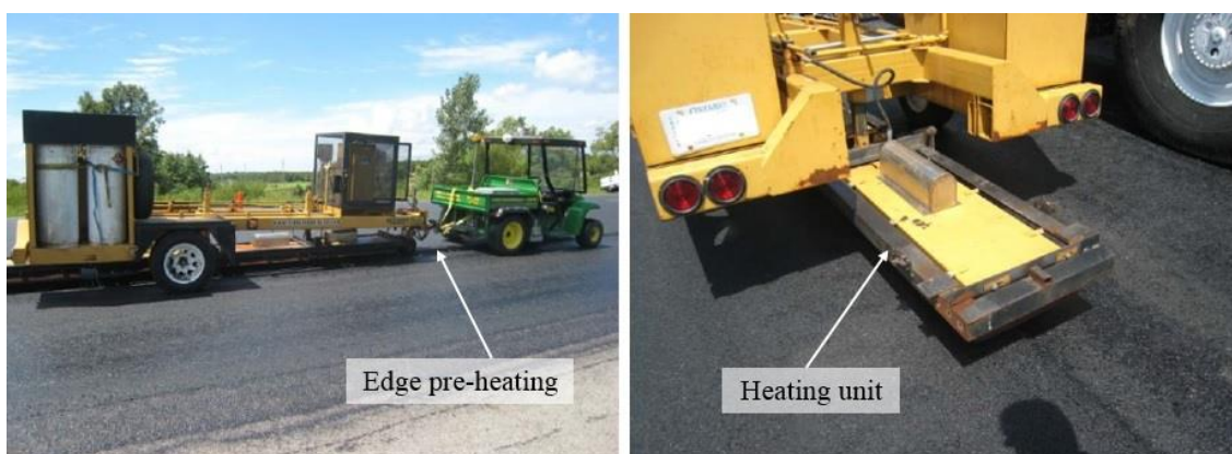
Figure 2.11 Heat Design Equipment, Inc. joint heater used in longitudinal joint adhesion by Huang et al. (2010) and Williams (2011) (images source Williams (2011, p.55), label added by author)
