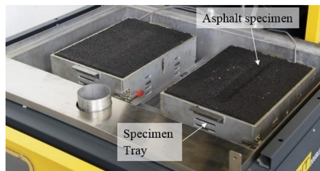
Figure 2.20 Demonstration of rectangular slab specimen and steel mould for wheel tracking test (Controls, 2018, p. n/a, label added by author)
