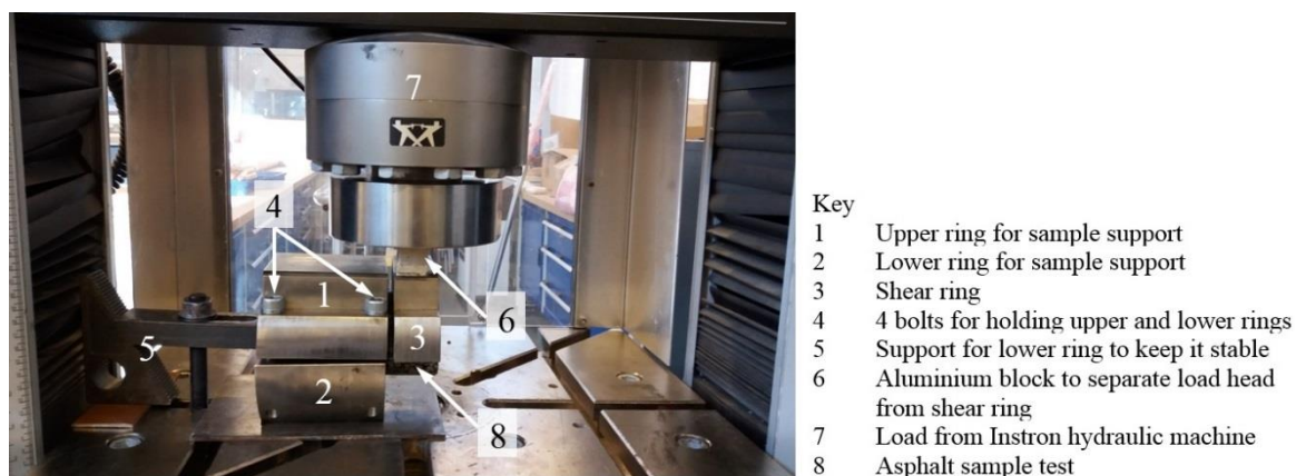
Figure 8.5 SBT apparatus designed for this study
