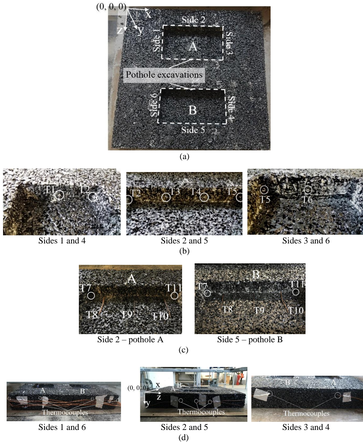
Figure 6.4 Thermocouples in static and dynamic repairs completed for pothole A and B respectively: (a) slab and coordinate system for Table 6.2; (b) thermocouples T1-T6 for measurement of temperatures in the vertical interfaces of the pothole repairs; (c) thermocouples T7-T11 for measurement of temperatures in the bottom of the pothole repairs; (d) thermocouple routes from pothole excavations to data loggers
