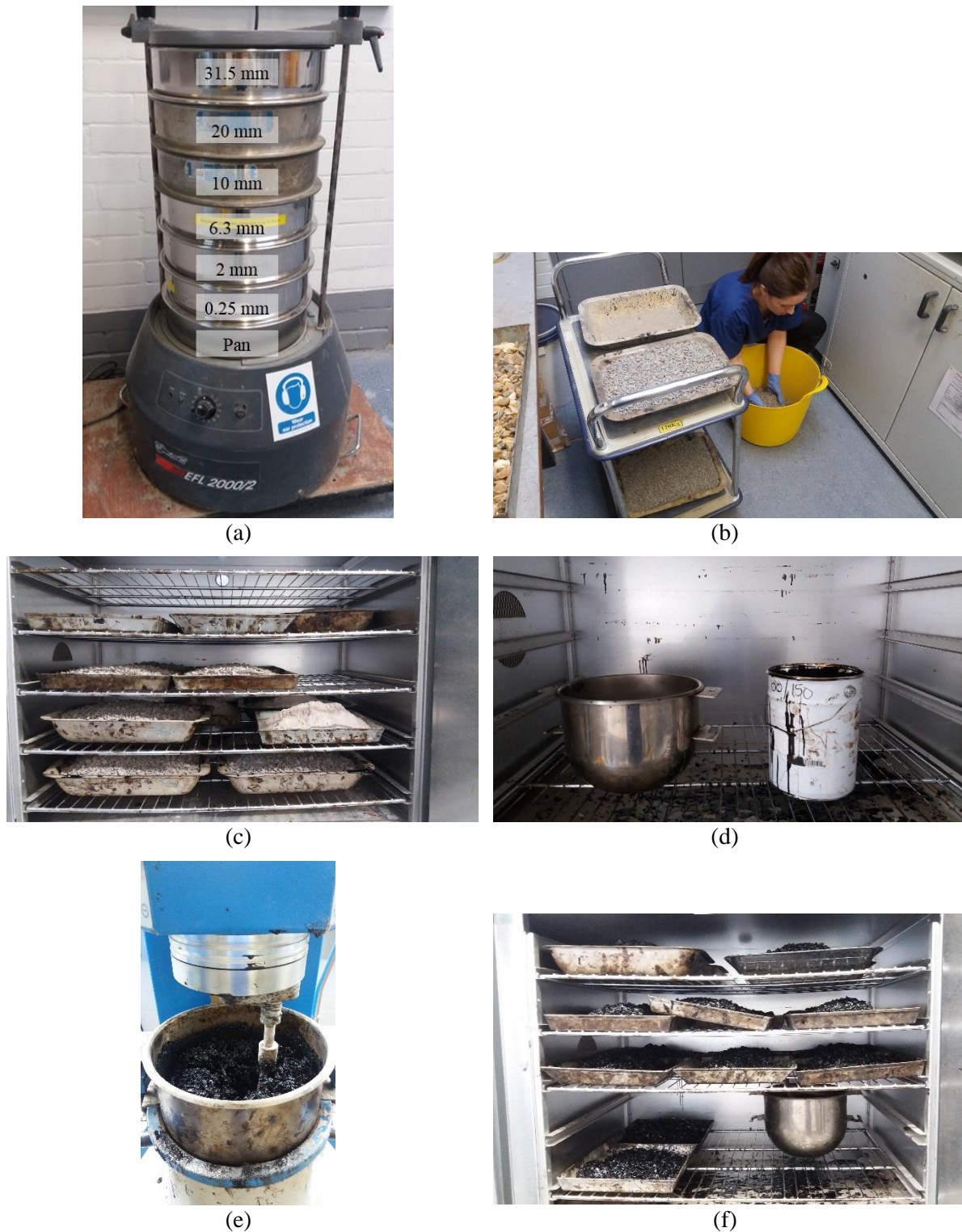
Figure 4.2 Preparation of HMA batches: (a) sieving; (b) manual mixing of aggregates; (c) drying and heating of aggregates and filler for (24 + 3) hours at 110 ( \pm 5 ) °C to a ventilated oven; (d) heating of binder and mixer bowl for 3 hours and 1 hour respectively at 140 ( \pm 5 ) °C to a ventilated oven; (e) mixing at 140 ( \pm 5 ) °C; (f) HMA
