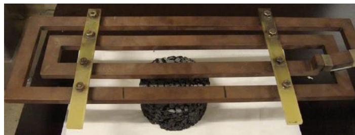
Figure 2.16 Common induction heating coil (Liu et al. , 2010, p.1209)
