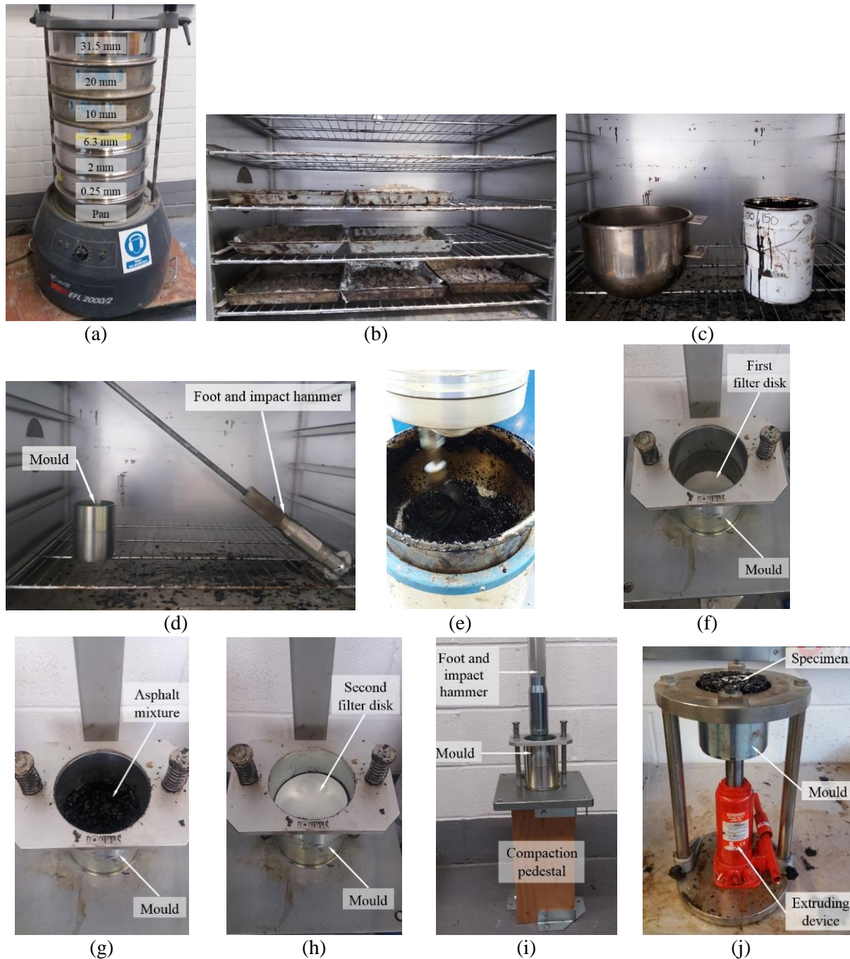
Figure 5.2 Preparation of test specimens: (a) sieving (example for 20 mm DBM mixture); (b) heating of aggregates and filler for 3 hours at 110 ( \pm 5) °C to a ventilated oven; (c) heating of binder and mixer bowl for 3 hours and 1 hour respectively at 140
