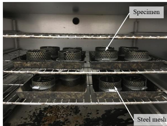
Figure 5.5 Conditioning of compacted specimen for 5 days at 85 ( \pm 3 ) °C to a ventilated oven for long-term ageing
