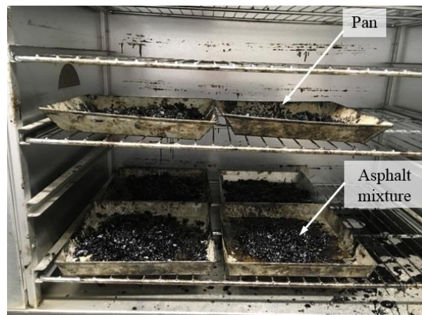
Figure 5.4 Conditioning of loose mixture for 4 hours at 135 (\pm 3) ^\circ\text{C} to a ventilated oven for short-term ageing
