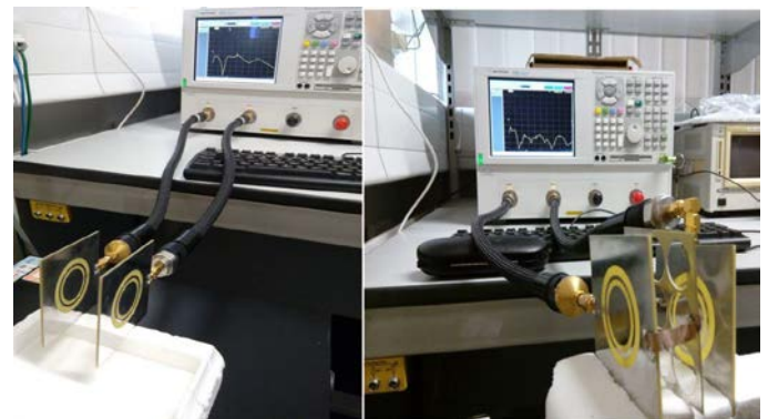
Fig. 4. Experimental setup for the reference (Right) and the proposed (Left) antenna array to measure the scattering parameters.
