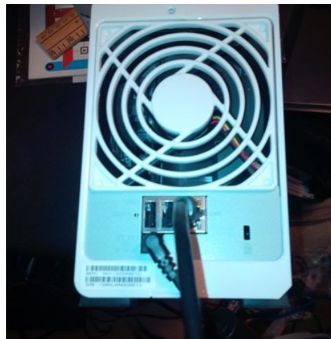
FIGURE 5.22: USB connection between NAS and G-Node
