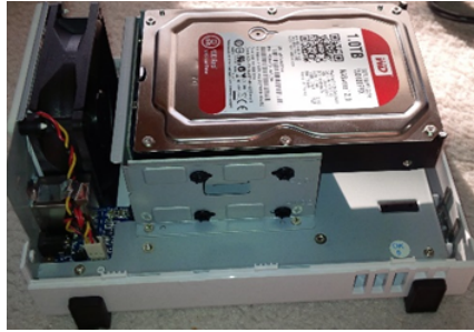
FIGURE 5.20: Multiple Bays system
