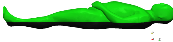
Figure 6: Top (green) and bottom (black) surfaces used to prescribe boundary conditions in whole body cooling
