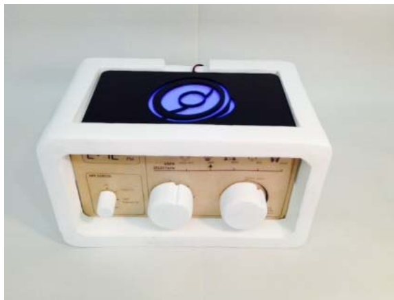
Figure 2 The prototype of the smart radio used in the study (see online version for colours)
