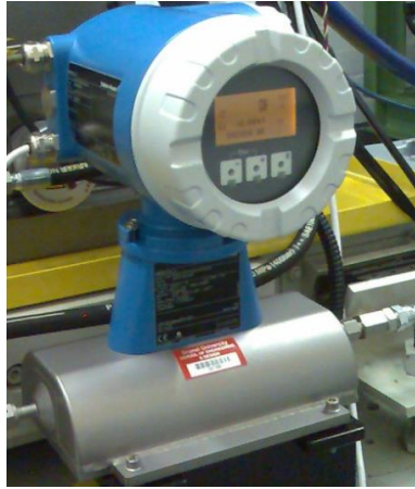
Figure 3.8 Endress+Hauser Coriolis Mass Flow Meter
