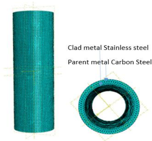
Fig. 2 (a) Full clad pipe showing quadratic tetrahedral elements of type C3D10 (b) Cross-section of pipe mesh showing clad metal and parent metal.
