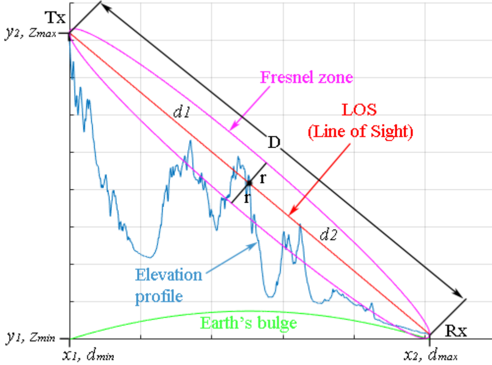
Figure 4-3: The first Fresnel zone.
