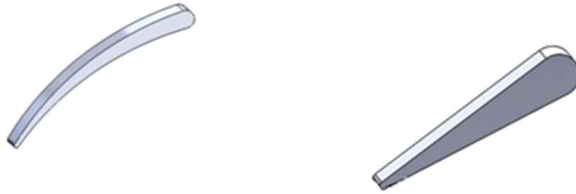
Figure 4-5: Configurations of stator vanes: cambered (left) and un-cambered (right).
