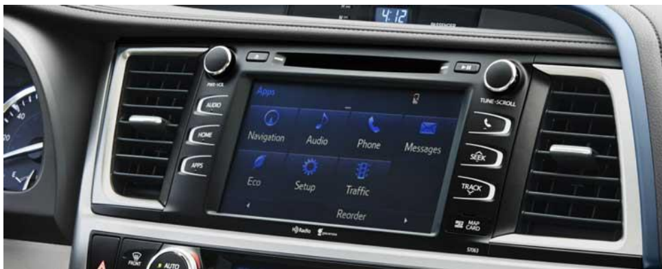
FIGURE 1.4 EXAMPLE OF A 2016 MODEL YEAR MULTIMODAL SCREEN BASED INFOTAINMENT SYSTEM USING A COMBINATION OF TOUCHSCREEN, 'HARD' BUTTON AND REMOTE CONTROL (TOYOTA CARS)
