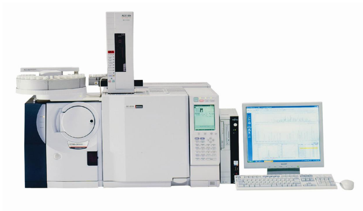
Figure 5. Photo of GC/MS analytical tool used for bio-oil analysis.
