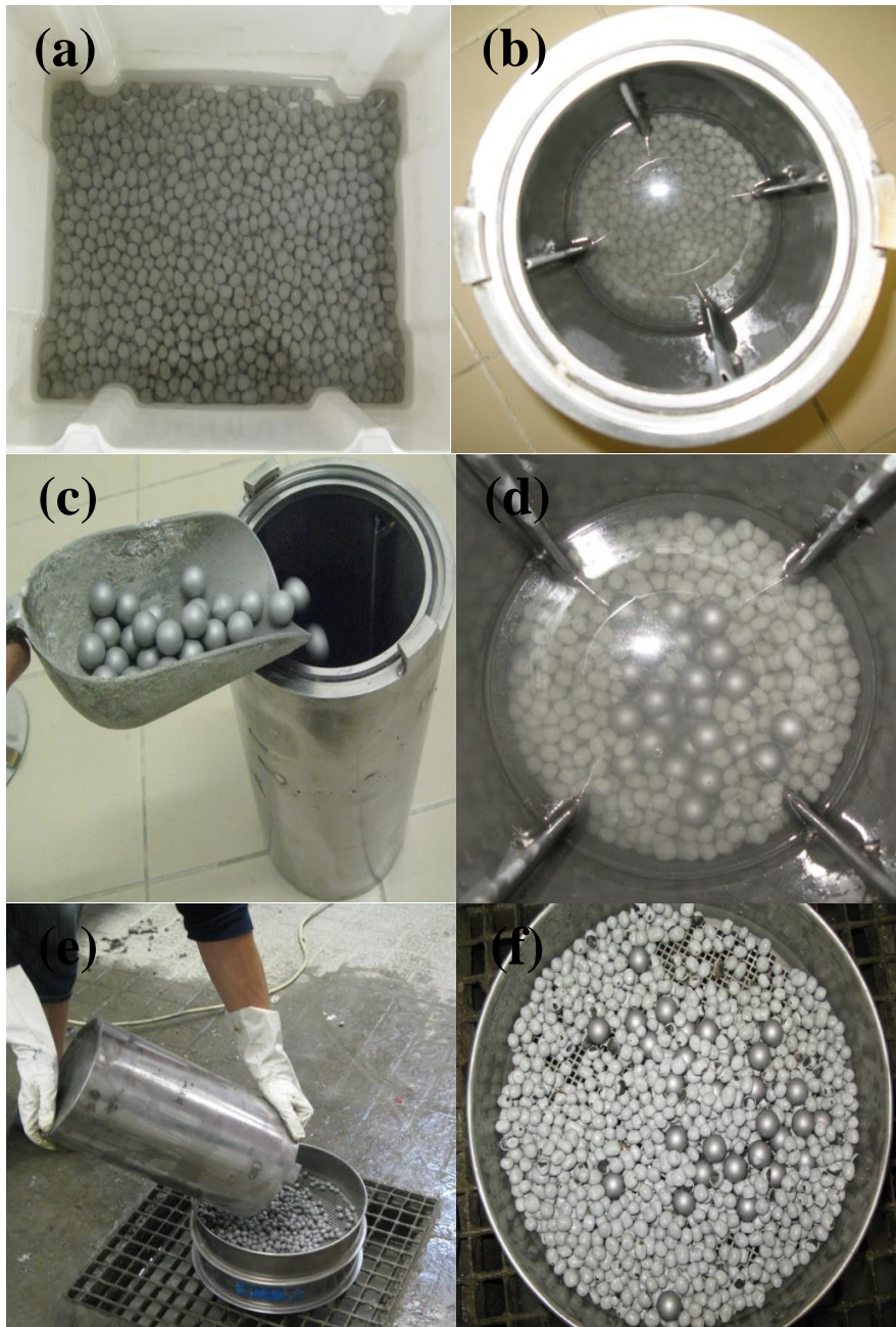
Fig. 5-18 test procedure to determine the ME-LWA durability showing (a) soaking the ME-LWAs (b) ME-LWAs in the drum (c) addition of the steel charge (d) ME-LWAs with steel charge in the drum submerged in water (e) removal of ME-LWAs after the test (f) separation of the ME-LWA from the steel charge
