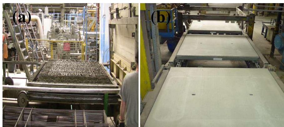
Fig. 2-4 Alkali-activated (a) fresh concrete and (b) final panel products developed by ASCEM (ASCCEM B.V., 2015)
