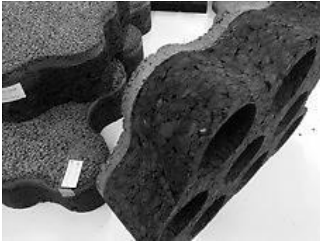
Fig. 2-9 GEOGREEN modules, consisting of an alkali-activated base plate using tungsten mining waste mud and an insulation corkboard
