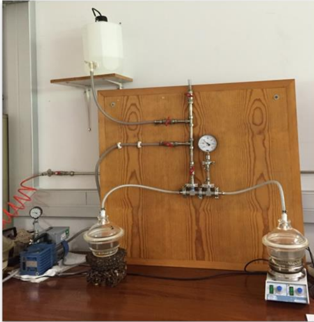
Fig. 5-2 LWA vacuum impregnation system
