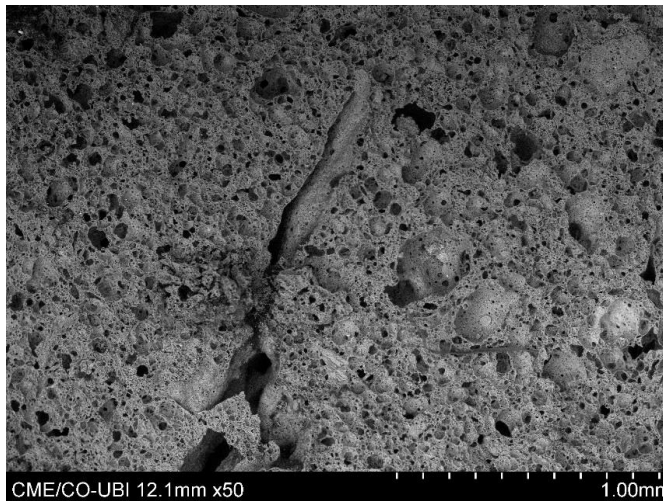
Fig. 5-1 x50 magnification SEM image of the LWA pore structure
