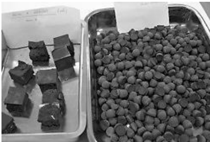
Fig. 2-8 Alkali-activated artificial aggregates produced from Panasqueira mining waste mud for wastewater treatment
