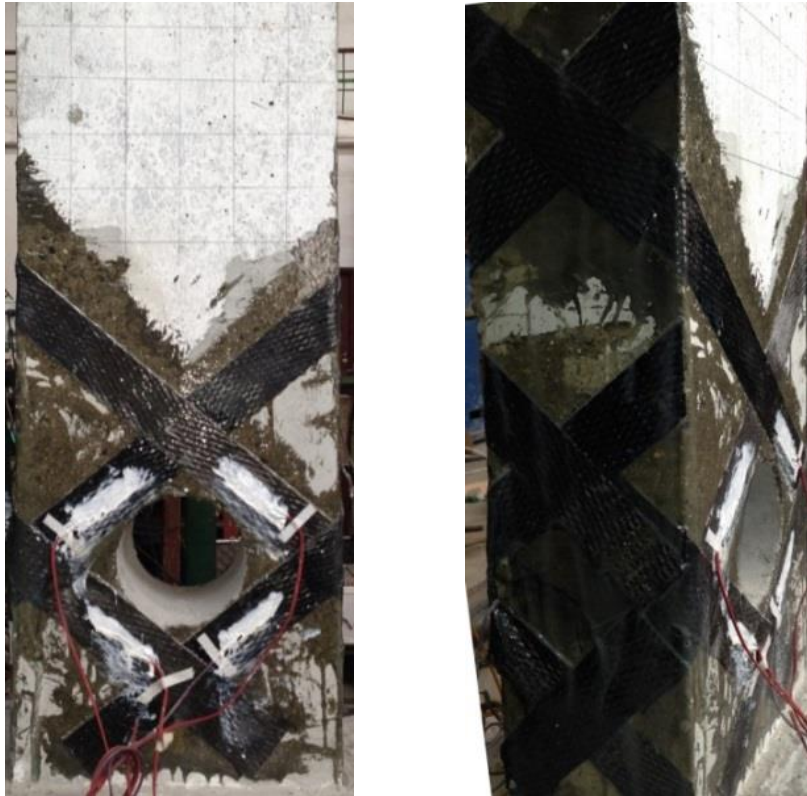
(b) Strengthening with 45° diagonal arrangement
