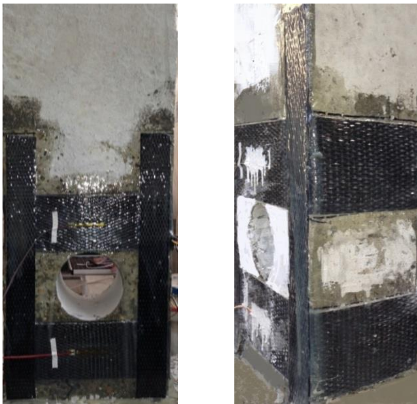
(a) Strengthening with horizontal arrangement
