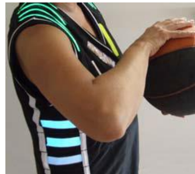
Fig. 2.3 Mitchell Page and Andrew Vande Moere (2007). 'TeamAwear' is a set of basketball jerseys with embedded electroluminescent wires
