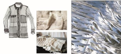
↑ The shirt Oricalco is composed by Shape Memory Alloy wires. The fabric forms itself into different shapes in response to the ambient temperature (Corpo Nove and Grado Zero Espace).
