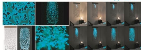
↑ Digital Dawn is a reactive window blind that digitally emulates photosynthesis using printed electroluminescent technology; a light-based botanical environment seems to grow on the window lamp as a room gets darker (Rachel Wingfield, 2011)
