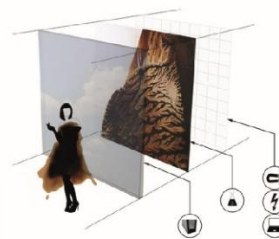
↻ Magnetism is used to allow façades to change translucency, colours and more. The idea behind Magnetic Architecture is to explore the possibility of producing a façade cladding that changes properties such as transparency, reflectivity, colour and even shape (Space Group Architects).
