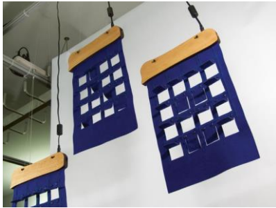
Fig. 2.4 Shutters' flaps have embedded SMA wires controlled with a circuit board concealed in the wooden panel. (Coelho et al. 2011)
