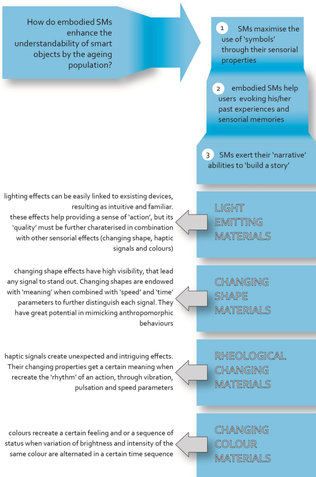
Figure 6.5 Flow chart explaining how embodied SMs enhance the understandability of smart objects by the ageing population and suggestions for future applications of the four SMs' families
