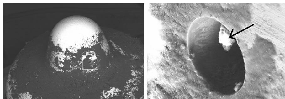
Fig. 2. Scanning Electron Microscopy images of a set 2 injector nozzle. Left image provides a full view of the nozzle, where deposits are clearly visible as black patches. Right image provides a magnified view of the orifice indicated by the white square in the left image, and where a deposit (black arrow) is clearly visible inside the hole.
