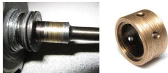
Figure 11: Shaft and bearing wear caused by contaminated oil [14]
