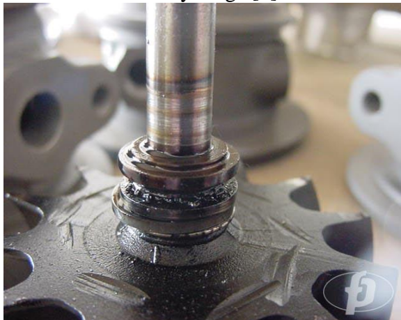
Figure 2: Charred oil residues accumulated in the piston ring region [1]
