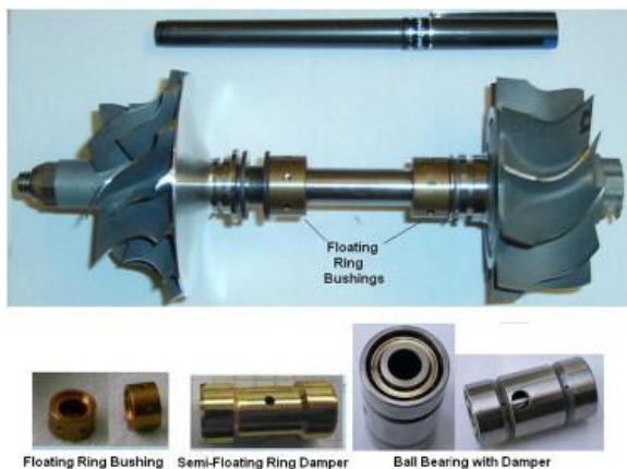
Figure 6: Different turbocharger bearing types with semi-floating dampering the middle [9]
