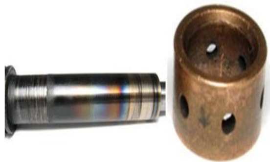
Figure 10. Shaft and bearing wear caused by the lack of lubrication. Shaft discoloring (bluing) is noticeable [13].
