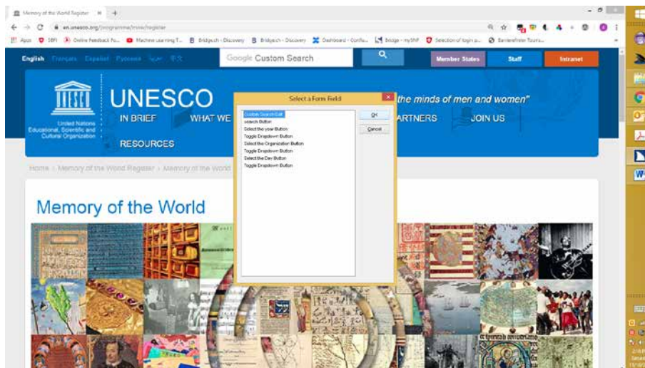
Figure 4. List of interactive form fields on the Memory of the World website, as shown by the screen reader program JAWS.
