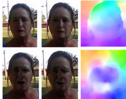
Figure 4.3 Samples of Optical Flow for consecutive frame
