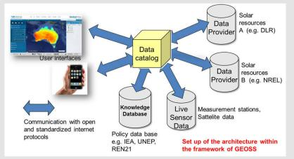
Concept of networked data bases in GEOSS applied to the Global Atlas of Renewable Energy Sources of IRENA. All data sources are registered in the data catalog and can be discovered there. Data sources provide standardized descriptions of access mechanisms, e.g., through WSDL (Web Service Description Language). Geo data is provided according to the standards of the Open Geospatial Consortium (OGC) Source: Own Composition.
