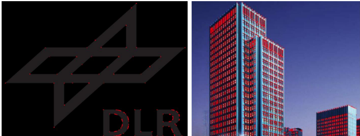
Figure 4.2: Successful detection of corners (red dots) using Harris Corner detector
